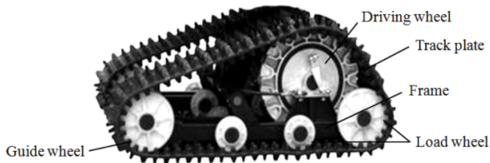
Fig. 1. Structure of a type of triangular track
