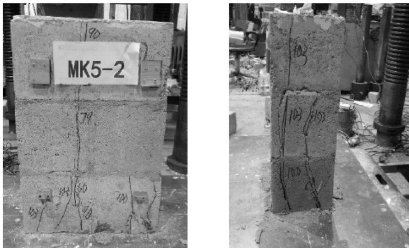
Fig. 4. Failure state of hollow compression standard parts
