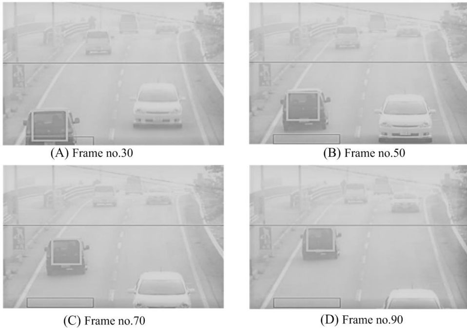
Fig. 5. Foggy and low speed vehicle tracking experiment result
