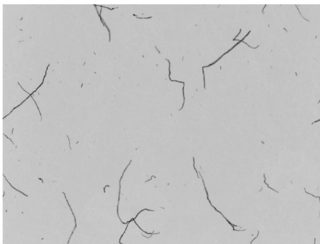
Fig. 2. Fiber morphology of the rayon grade pulp
