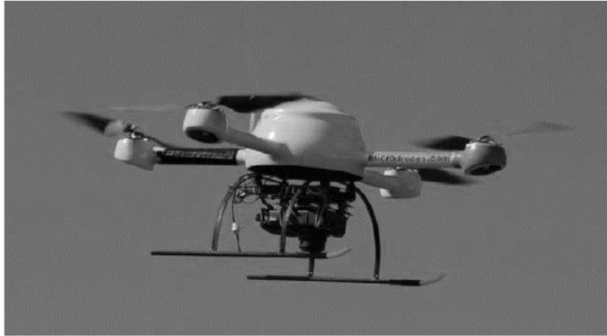
Fig. 1. Microdrone md4-200 with a Ricoh GR3 compact camera
