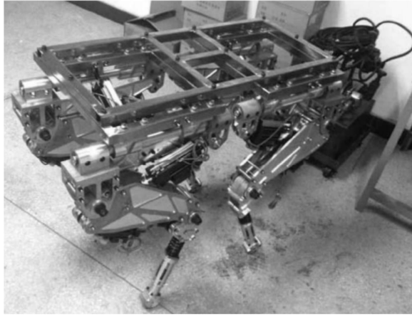
Fig. 3. Principle prototype of quadruped robot
